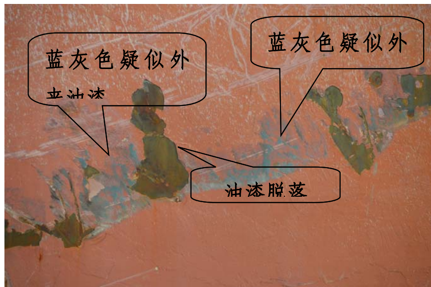
图9/10: “SILVER PHOENIX”轮球鼻艏左侧遗留凹陷和痕迹
